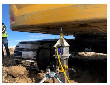
Figure 4-3: Axial Compressive Testing Example
