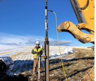
Figure 4-1: Axial Tensile Testing Example
