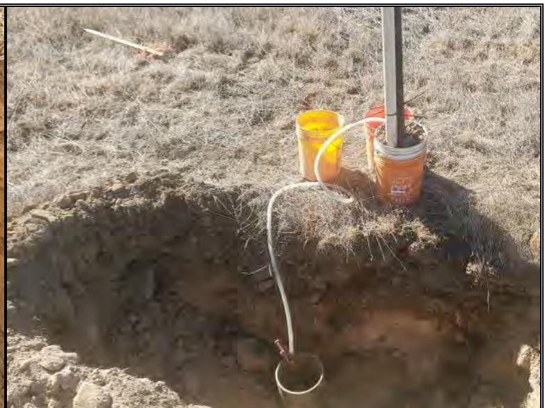
Infiltration test setup at P-1
