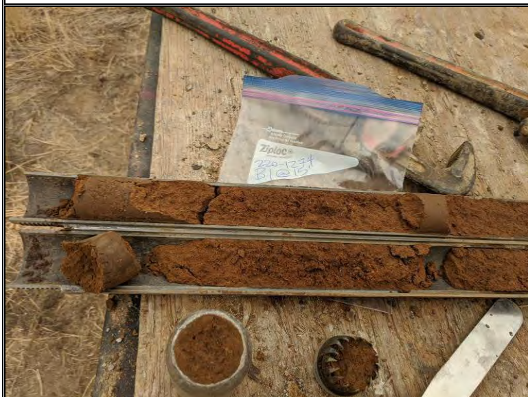
Split-spoon sample obtained from boring B-1 at 15' BGS
