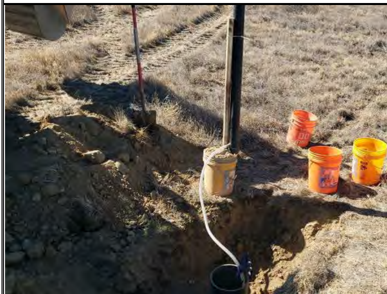
Infiltration test setup at P-3
