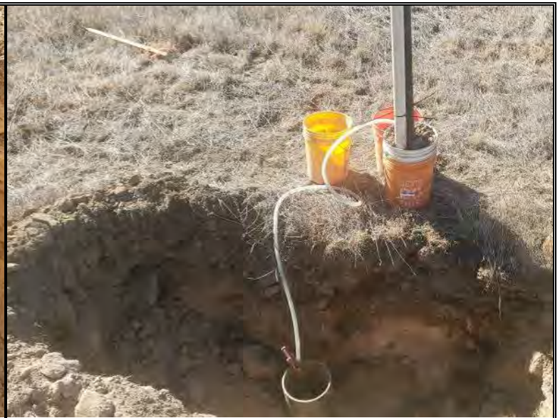
Infiltration test setup at P-1
