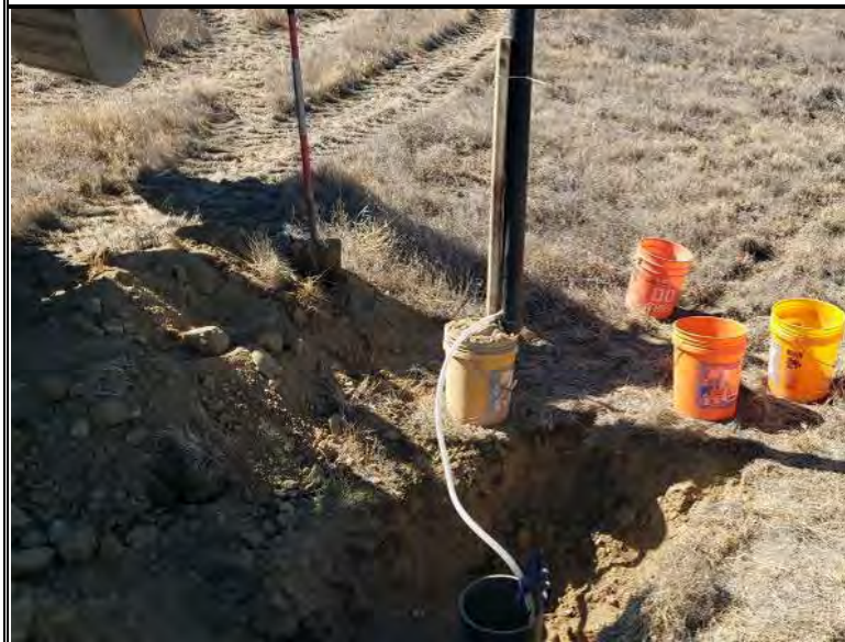
Infiltration test setup at P-3
