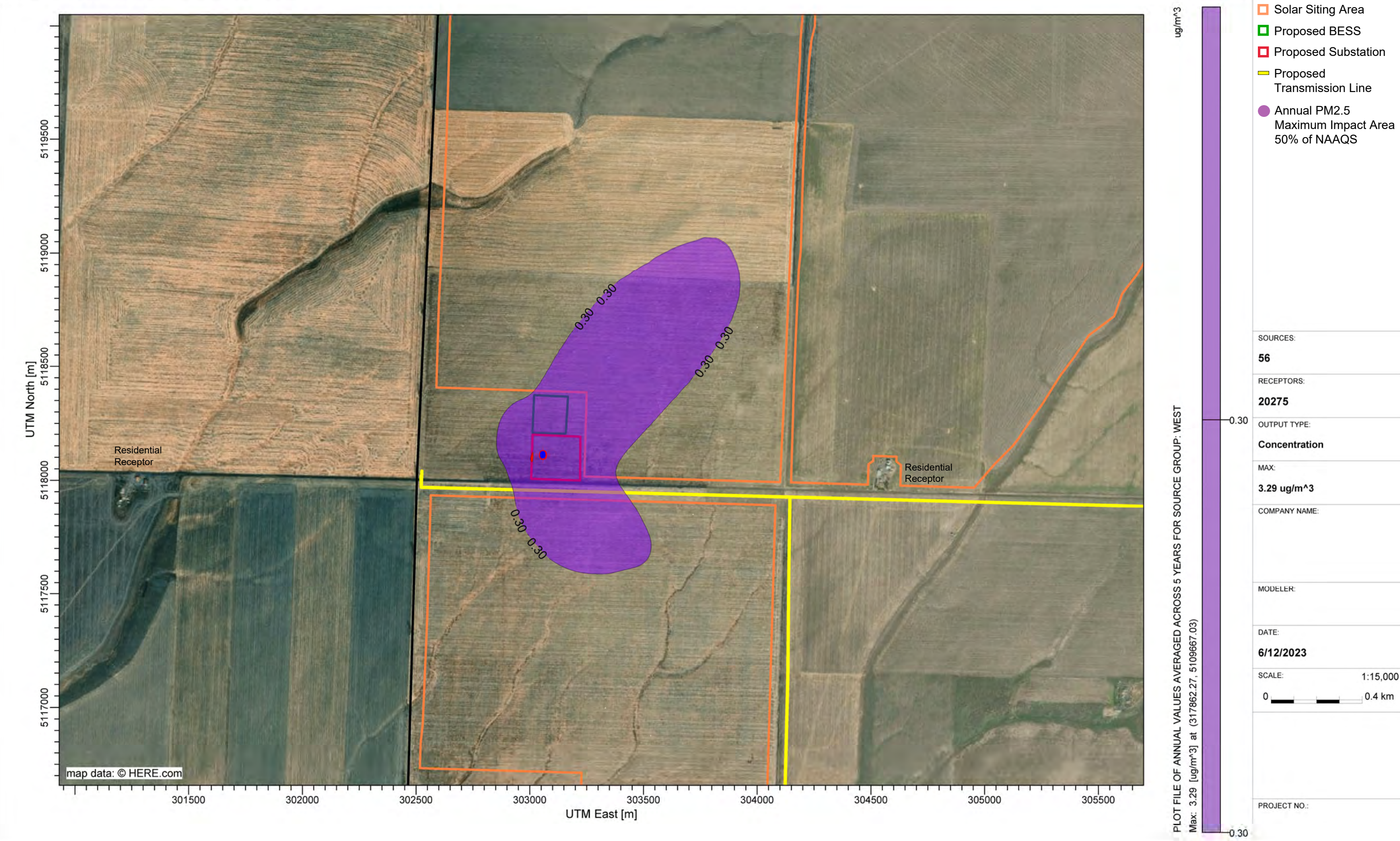
Figure C-10 Horse Heaven - Air Quality Dispersion Modeling Evaluation Stationary Engines - West Substation - Annual PM2.5
