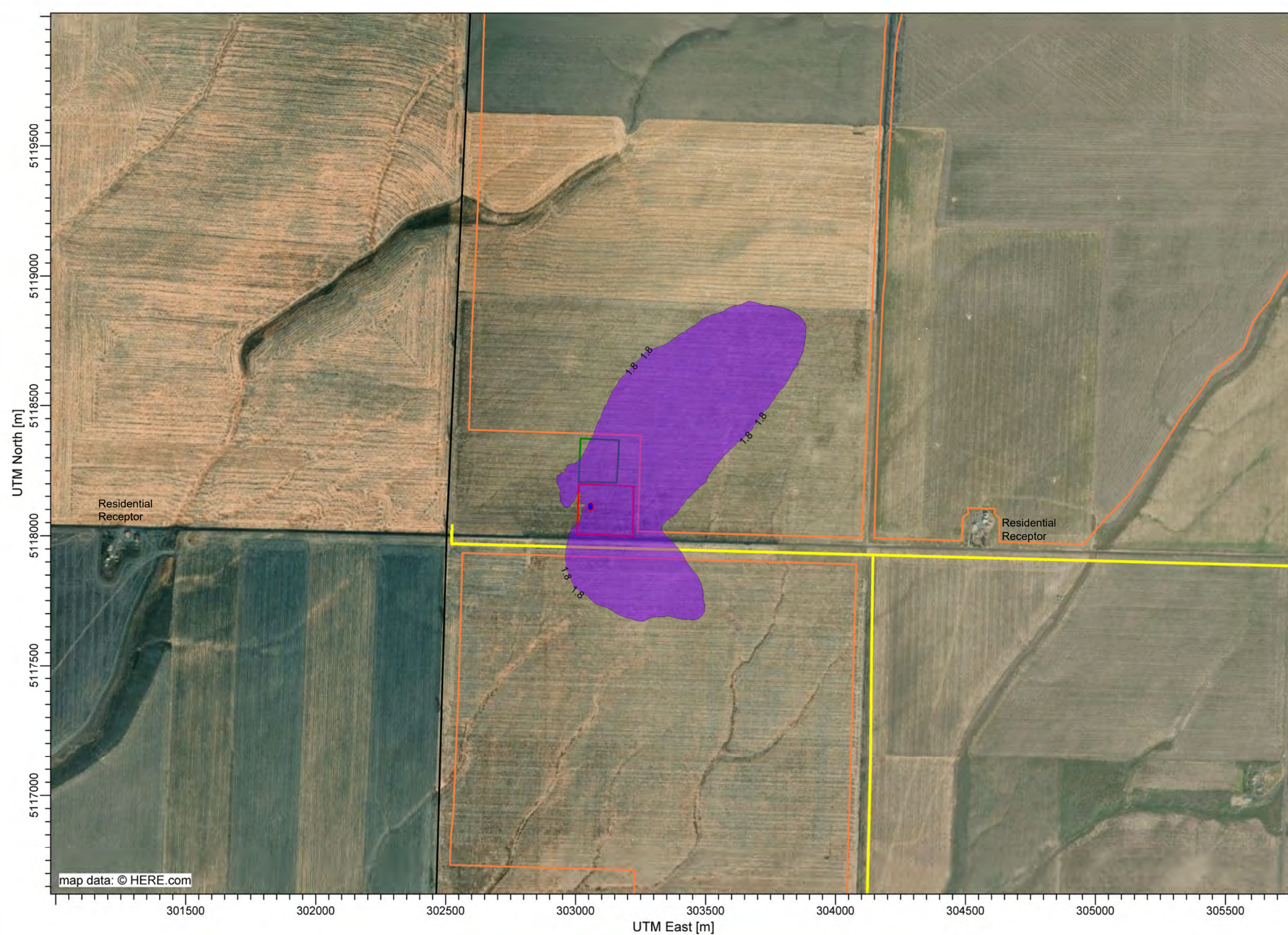
Figure C-5 Horse Heaven - Air Quality Dispersion Modeling Evaluation Stationary Engines - West Substation - 24-hour PM2.5
