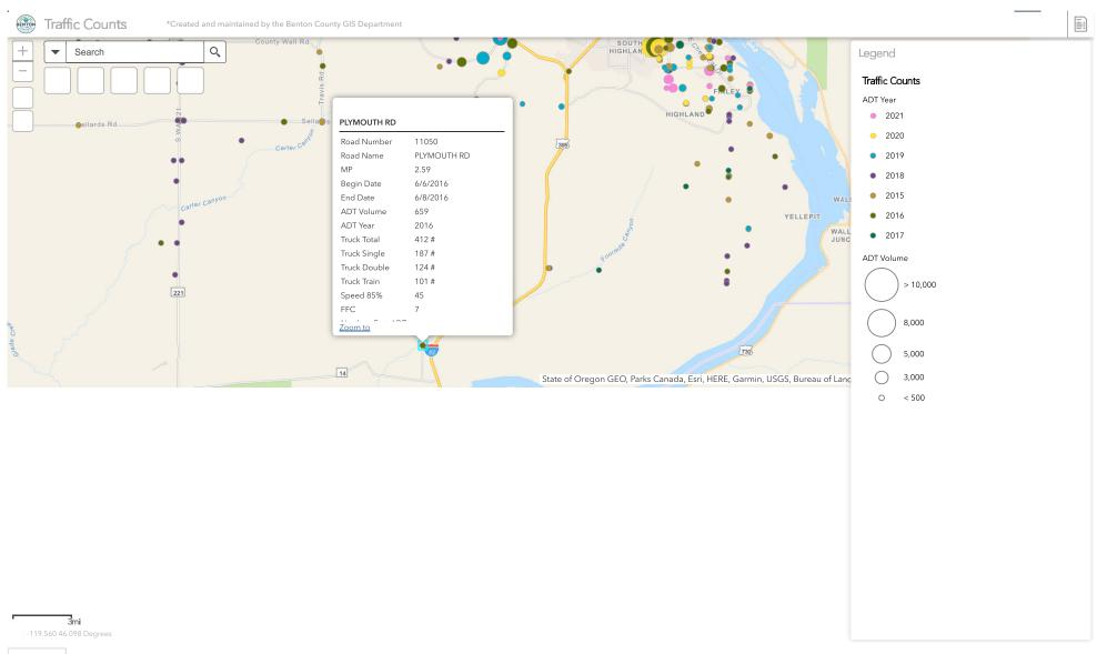
Traffic Counts Options Filter by map extent Zoom to Clear selection Refresh Road\_Number Road\_Name Begin\_Date End\_Date ADT\_Volume ADT\_Year Truck\_Total Truck\_Single Truck\_Double Truck\_Train Speed\_85% North or East South or West 412# 11050 PLYMOUTH RD 2.59 6/6/2016 6/8/2016 659 2016 187# 124# 101# 45
