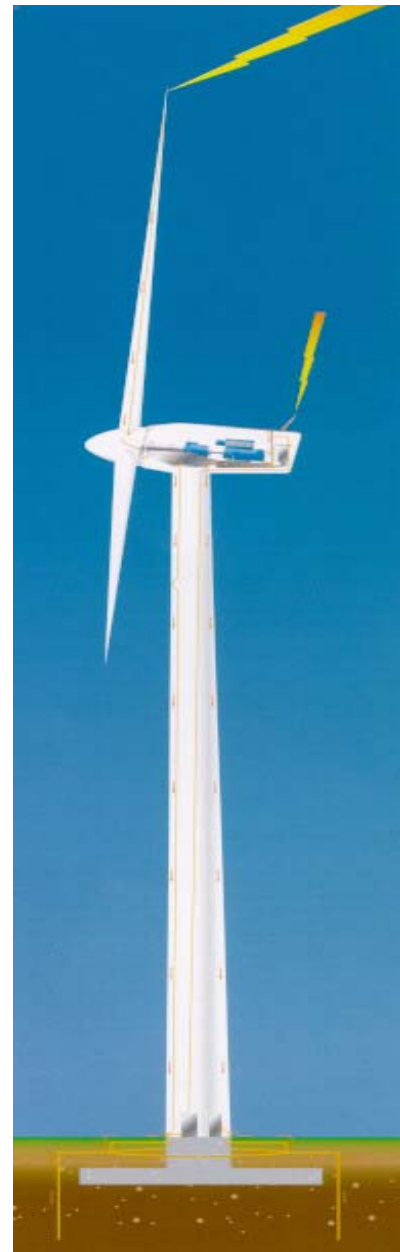
Figure 2.2.3.6-2 WTG Lightning Diversion Paths
