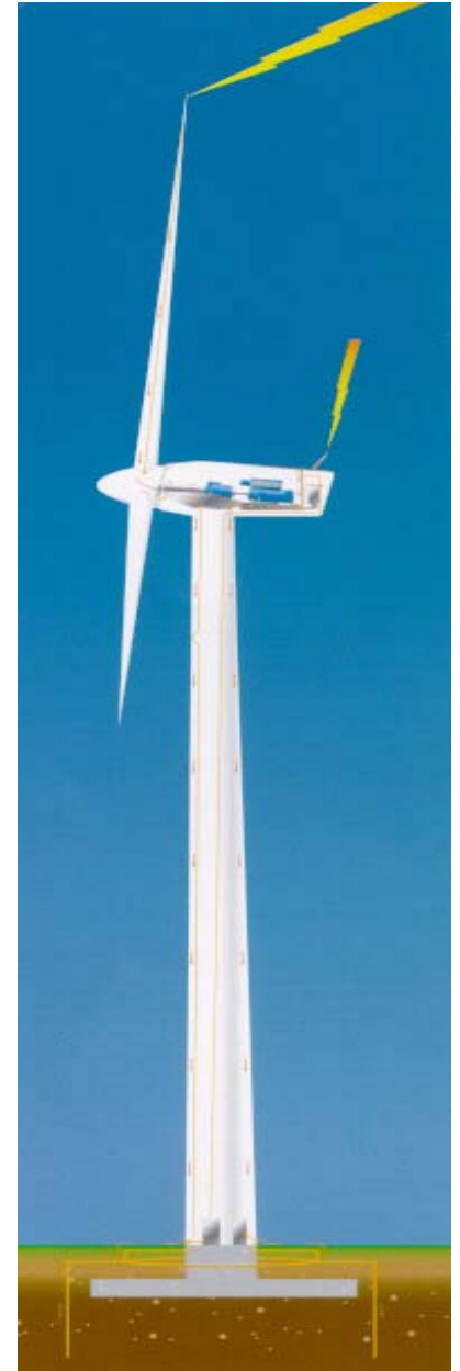
Figure 2.3.6-5 WTG Lightning Diversion Paths
